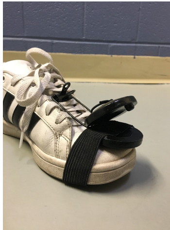
Figure 2: Shoe with Clipper Clapper attached
